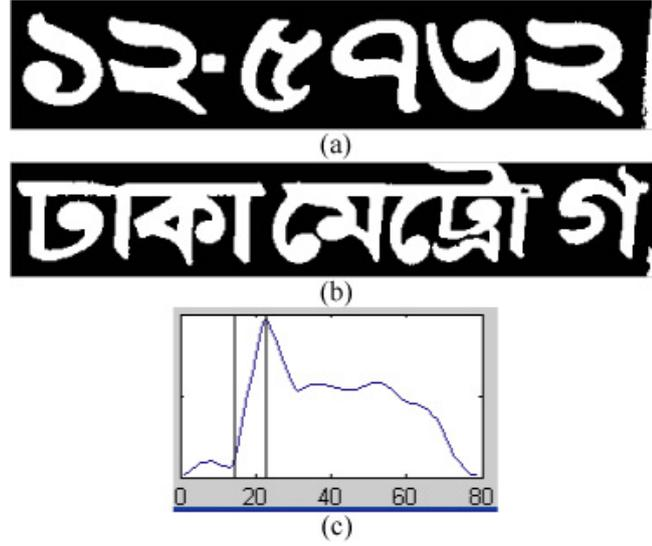
Fig. 4.4: Threshold initialization step: (a) Separated row containing digits, (b) Separated row containing characters, and (c) Calculating initial threshold.
