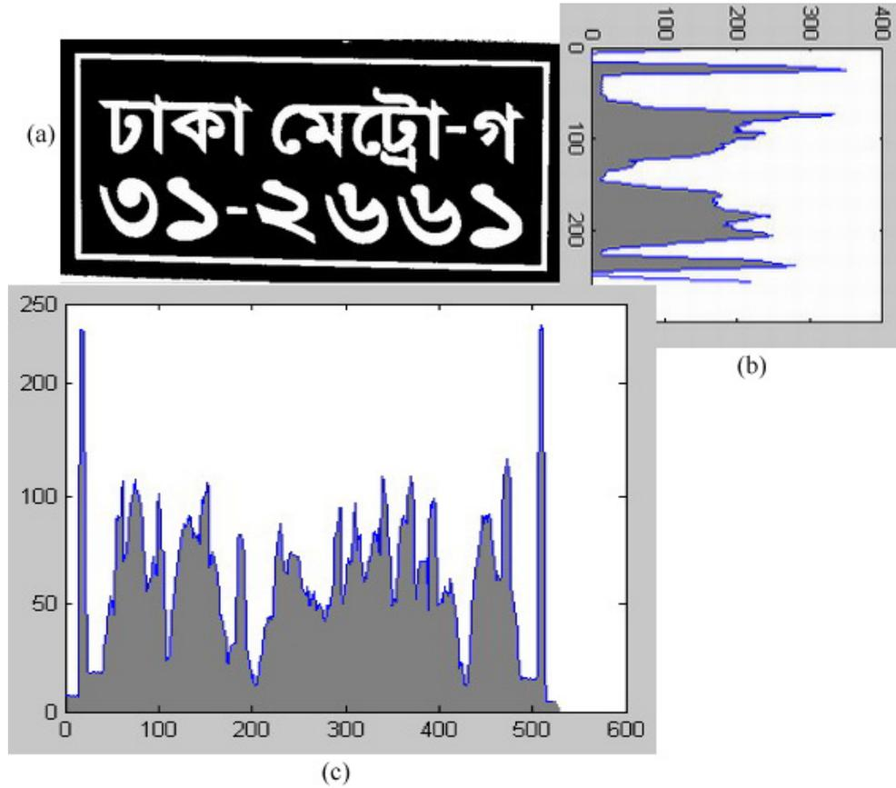
Fig. 2.6: (a) Original license plate image, (b) Horizontal projection, and (c) Vertical projection.
