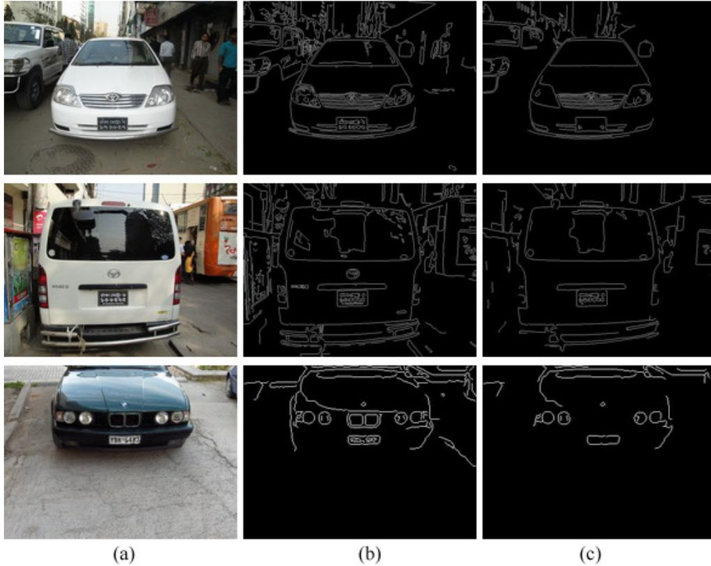
Fig. 2.2: (a) Original input images, (b) Canny edge images (threshold = 0.5), and (c) Canny edge images (threshold = 0.3).
