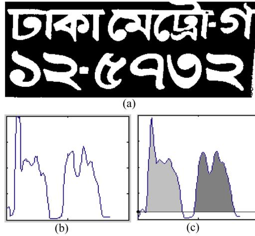
Fig. 4.2: Sample outputs of license plate segmentation stage: (a) Binary image of a simple license plate, (b) Horizontal projection of the pixels, and (c) Filtered projection.
