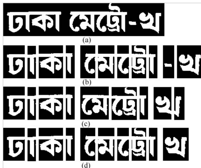
Fig. 5.2: Character segmentation: (a) Original license plate, (b) Manual segmentation, (c) Segmentation with constant threshold [4], and (d) Segmentation with adaptive threshold (Algorithm SAT).
