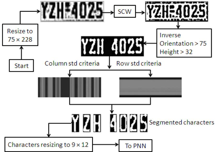
Fig. 3.2: Flowchart indicating the license plate segmentation process [3].
