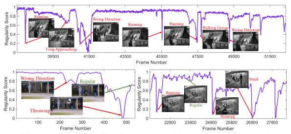
Figure 11. Regularity score (Eq.3) of each frame of three video sequences. (Top) Subway Exit, (Bottom-Left) Avenue, and (Bottom-Right) Subway Enter datasets. Green and red colors represent regular and irregular frames respectively.
