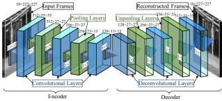
Figure 4. Structure of our fully convolutional autoencoder.
