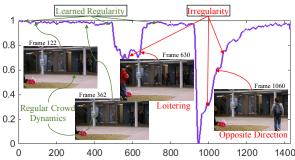
Figure 1. Learned regularity of a video sequence. Y-axis refers to regularity score and X-axis refers to frame number. When there are irregular motions, the regularity score drops significantly (from CUHK-Avenue dataset [8]).
